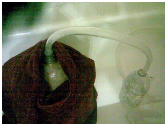
Barley Wine with blow-off applied just before the foam reached the airlock. By 3am the foam had overflowed the blow-off bottle (right) which got switched out with the priming bucket.
